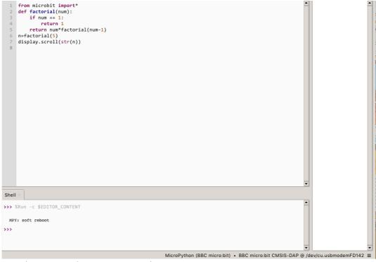
Figure 4: The Factorial Function in Python using Recursion
