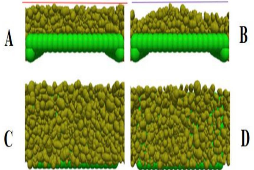
Figure 1: Deposited Powder Layers during the Simulations of Powder Spreading. Adapted from (1).
